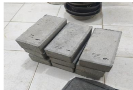
Gambar 8. Paving Block Tanpa Campuran
